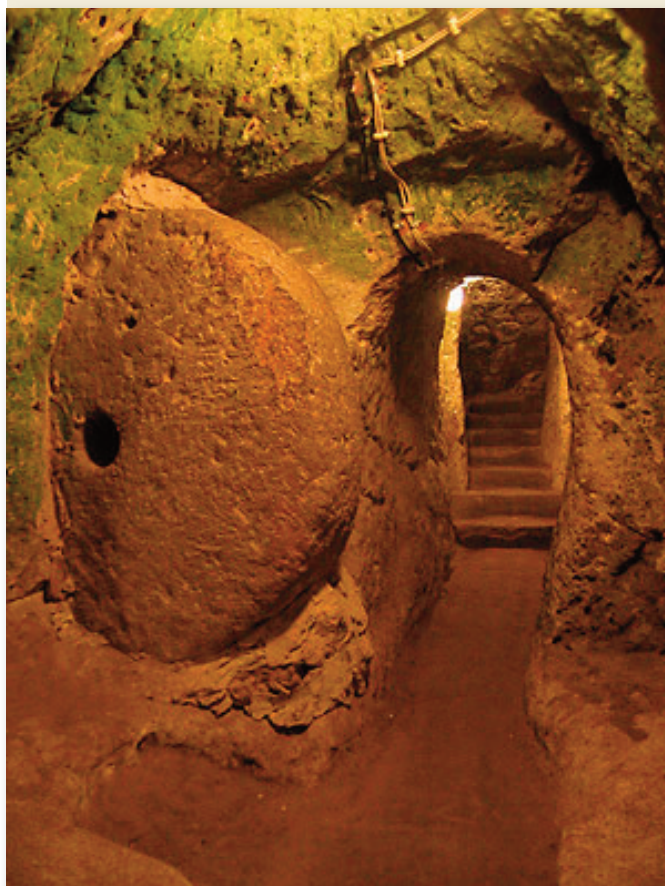
Below: Carefully balanced moving stone doors, resembling mill stones, were devised to quickly block the corridors in the event of an attack. (Photo: goreme.com)
